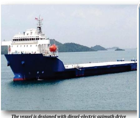
The vessel is designed with diesel-electric azimuth drive propulsion system for efficiency maneuverability and lower fuel consumption. It is installed with DP2 and has a heavy deck load design of 20T/M2 with point loads of up to 300T.
