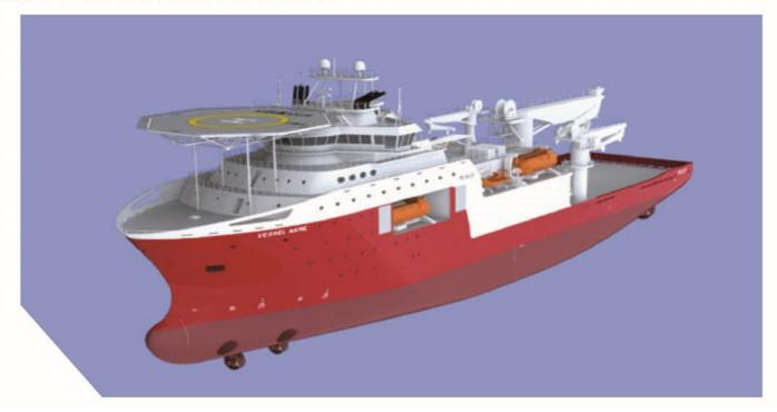
The vessel is an advanced deep sea offshore vessel intended to operate in most weather conditions all over the world and with good maneuverability and station keeping capabilities. The vessel will also be designed for relatively high transit speed.
